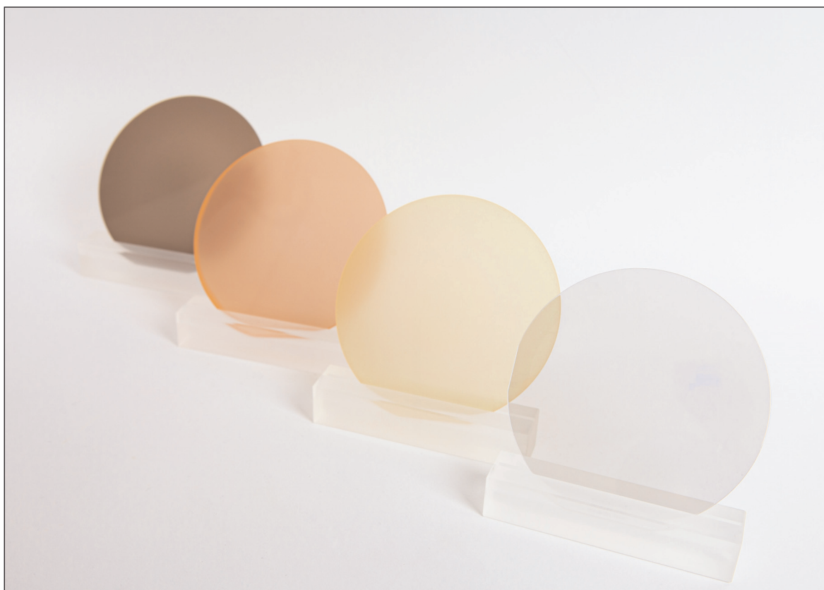
The different color nuances of the AlYN/GaN wafers result from different yttrium concentrations and growth conditions. © Fraunhofer IAF.
