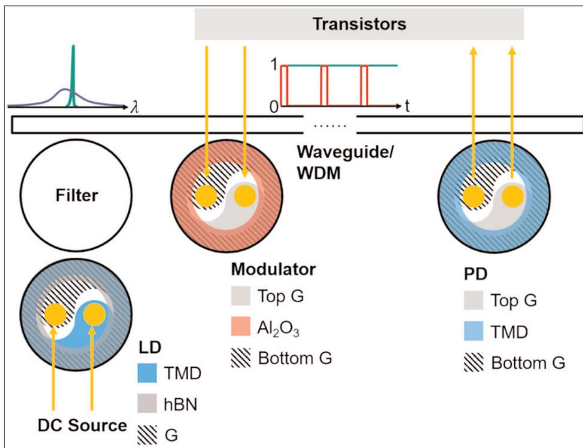
**Figure 2. Integrated photonic circuits with hBN disk cavity and waveguide on SiO<sub>2</sub>/Si platform.**
