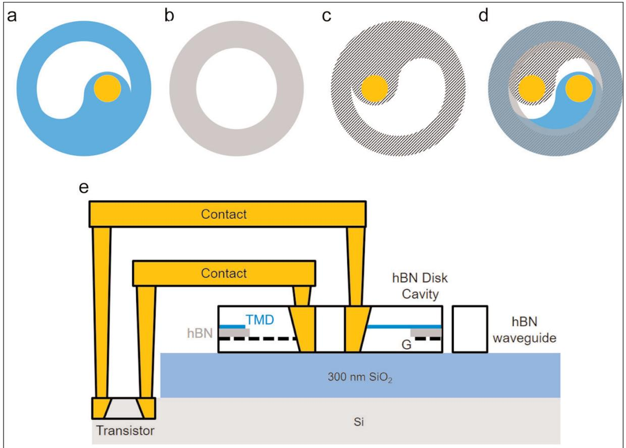
**Figure 1. Schematic design of proposed LED with hBN disk cavity. Top view patterns of (a) top TMD layer, (b) middle hBN layer, (c) bottom graphene (G) layer, and (d) TMD/hBN/graphene trilayer; (e) side view of LED structure connected with silicon transistor.**
