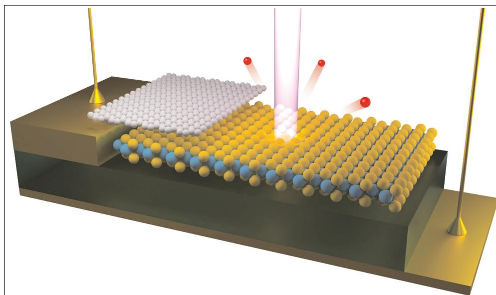
**Figure 3. Electrons ejected by a beam of light focused on two-dimensional semiconductor device are collected and analyzed to determine how electronic structure in material changes as voltage is applied between electrodes. Credit: Nelson Yeung/Nick Hine/Paul Nguyen/David Cobden.**
