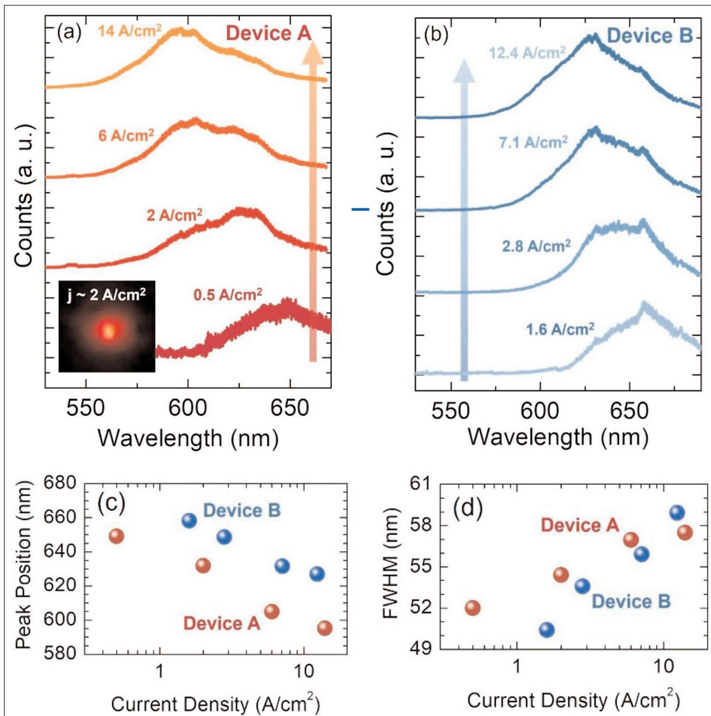
**Figure 3. Electroluminescence (EL) spectra with various injection currents for devices (a) A and (b) B. Inset: (a) image of device under operation. (c) Peak position and (d) full-width at half-maximum (FWHM) versus current density.**
