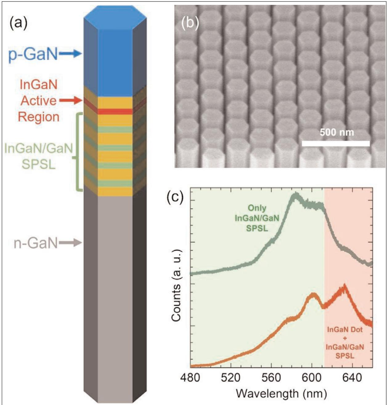
**Figure 2. (a) Schematic of N-polar InGaN/GaN nanowire LED heterostructure. (b) Scanning electron microscope image of N-polar nanowire array. (c) Photoluminescence (PL) spectra of nanowires grown with and without InGaN dot, showing red emission from InGaN dot.**
