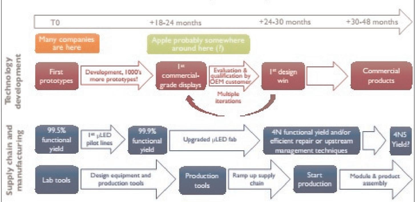
discrete micro-driver ICs have been developed by X-Display. The multiple prototypes based on TFT backplanes give credence to the idea that micro-LED displays could leverage existing panel makers' capacity, simplifying and streamlining the supply chain. "Equipment makers have taken notice and are starting to develop micro-LED-specific tools for assembly,
