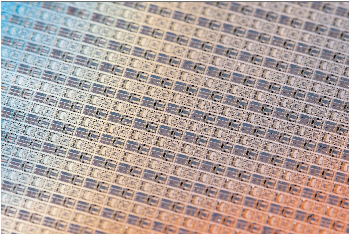
**High-frequency amplifiers based on aluminium scandium nitride (AlScN) have the potential to significantly improve the power density and efficiency of high-frequency amplifiers in 5G base stations. © Fraunhofer IAF**
