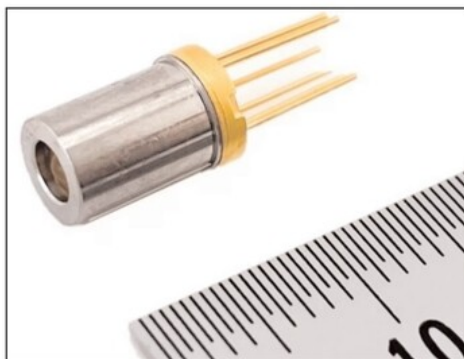
The ML973A71 DFB-CAN with built-in wavelength monitor.
