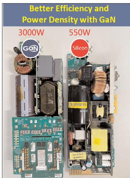
**3000W GaN power supply versus 550W silicon power supply (Xuzhou GSR Semiconductor Co Ltd).**
