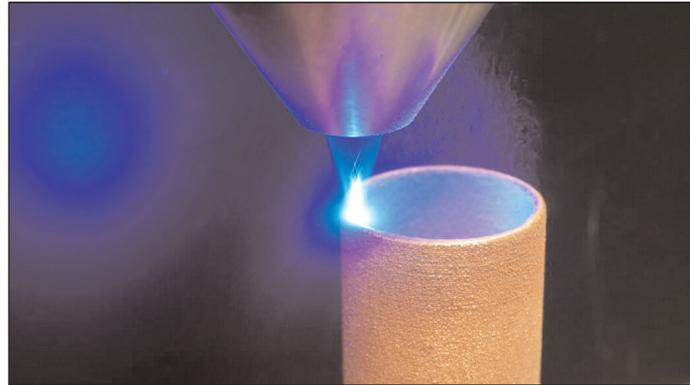
infrared radiation, this spectral range is absorbed much better by non-ferrous metals such as copper and gold. Among other benefits, this allows the heat conduction welding of copper components close to the surface, along with more energy-efficient and climate-friendly processes.
