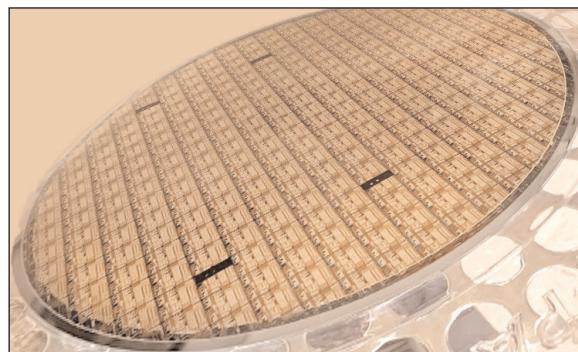
As a result, CEA-Leti's GaN/Si technology performance at 28GHz is gaining ground on GaN/SiC technology in terms of power density.
