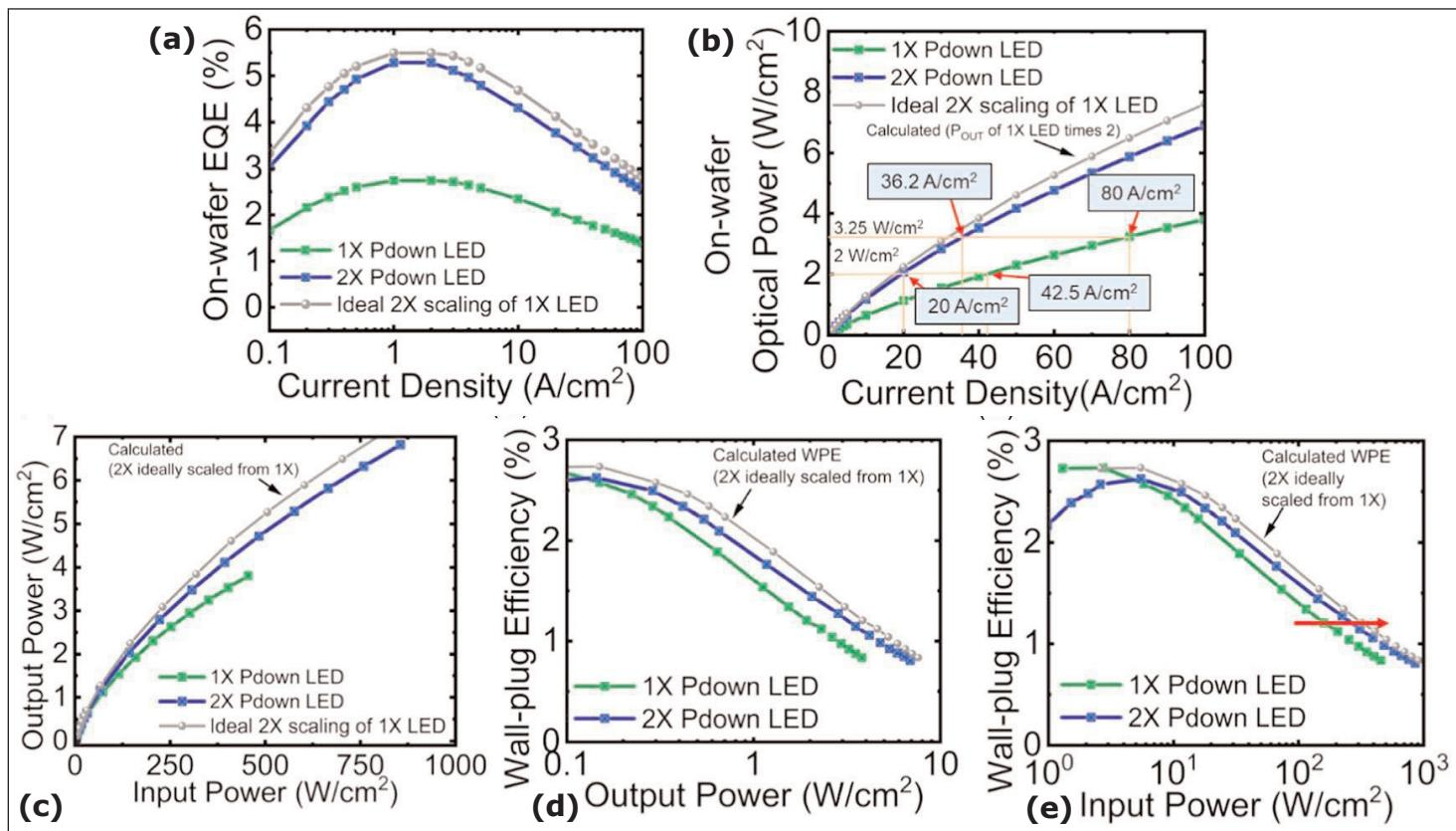
**Figure 2. (a) On-wafer measured EQE for single-junction and dual-junction devices. (b) Optical power. (c) Electrical input power and output optical power. (d), (e) Calculated wall-plug efficiency with corresponding output power and input power.**
