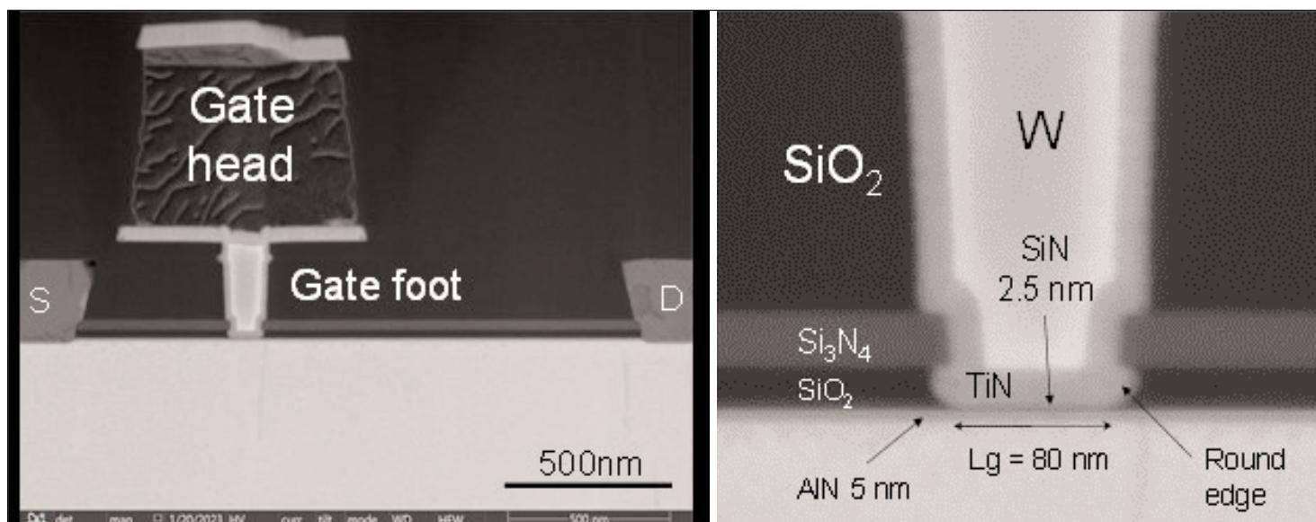
Scanning transmission electron microscopy cross section of the AlN/GaN MIS-HEMT and zoom on the gate foot.
