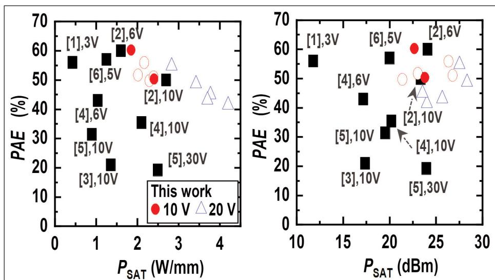
**Large-signal performance benchmarking (at 28–40GHz) for gallium nitride MISHEMTs, MOSHEMTs and AlN/GaN HEMTs integrated on a silicon substrate.** The graph shows PAE versus  $P_{SAT}$  normalized with gate width (W/mm). [1] H. W. Then, IEDM, pp402-05, 2019; [2] H. W. Then, IEDM, pp230-233, 2021; [3] P. Cui, Semi. Sci. Tech., 38 035011, 2023; [4] H. Du, EDL, vol.44, no.6, pp911-14, 2023; [5] E. Carneiro, Electronics, 12(13), p2974, 2023; [6] H. W. Then, VLSI 2020.
