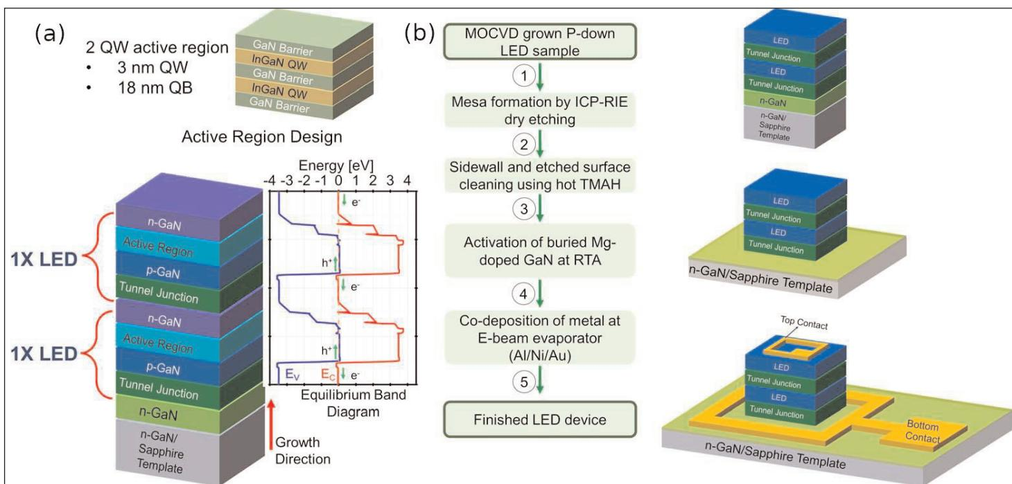
**Figure 1. (a) Epitaxial structure of dual-active-region p-down LED with active region design and corresponding equilibrium band diagram. (b) Process flow for single-junction and dual-junction p-down LEDs.**
