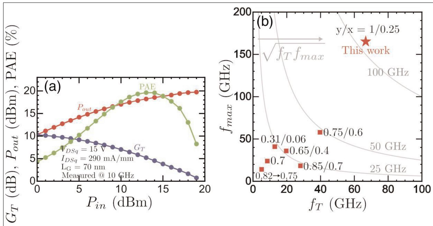
**Figure 2. (a)** RF power sweep at 10GHz at  $V_{DSq}/V_{GSq} = 15/-3$ V. **(b)** Benchmark comparing  $f_T/f_{max}$  of AlGaN-channel HEMTs reported in literature and Cornell's latest work.  $y/x$  indicates the aluminium composition in the top barrier/channel layer ( $\text{Al}_y\text{Ga}_{1-y}\text{N}/\text{Al}_x\text{Ga}_{1-x}\text{N}$ ).
