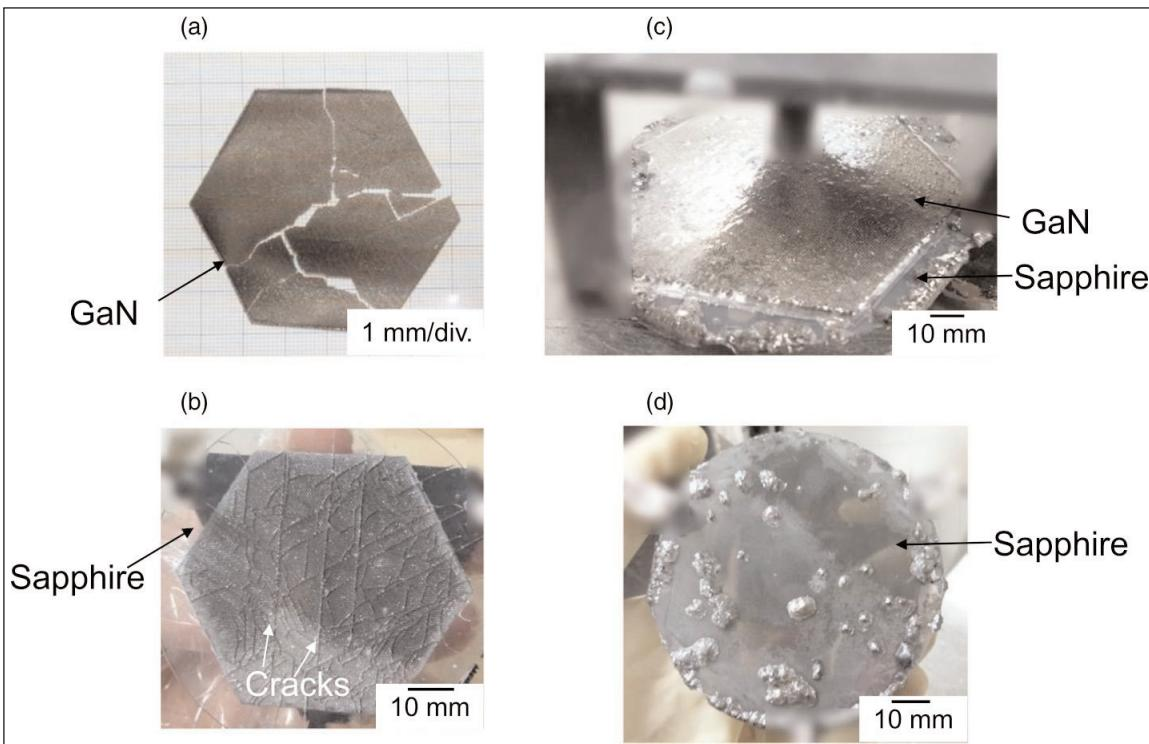
**Figure 2. Optical images of grown crystal (a) on MPS substrate viewed from GaN surface and (b) viewed from sapphire surface; (c) grown crystal on LAS-MPS substrate viewed from GaN surface and (d) from sapphire surface.**
