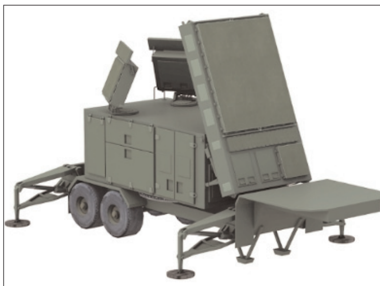
Artist's rendering of Raytheon's 360° capable Patriot radar array enhanced with GaN-based AESA technology. Raytheon's Patriot is owned by 13 nations, and has more than 200 combat engagements, 1400 flight tests, and 3000 ground tests.
