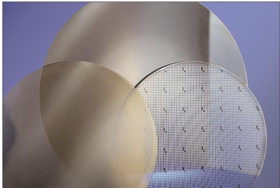
**Silicon carbide epi and wafer.**
