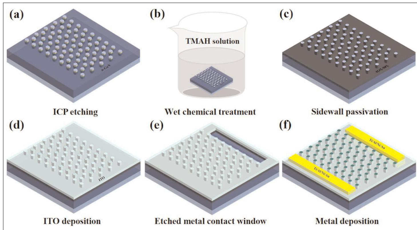
**Figure 1.** Process flow of cyan-green GaN-based QD micro-LED array: (a) ICP etching, (b) wet chemical treatment, (c) sidewall passivation, (d) ITO deposition, (e) etched metal contact window, and (f) metal deposition..
