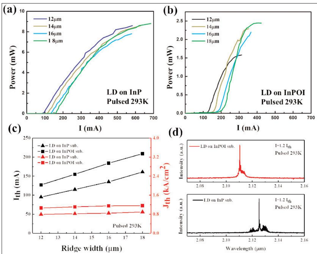
**Figure 2. Lasing properties at 293K with different ridge widths on (a) InP and (b) InPOI under 5% duty cycle, 2kHz pulsed mode; (c) threshold current/current density versus ridge width; (d) lasing spectra for 14μmx1mm ridges.**
