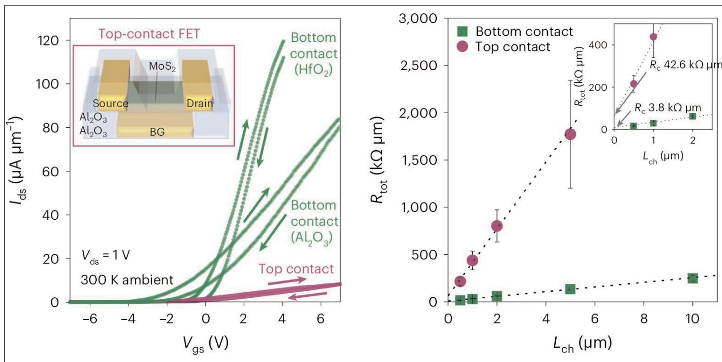
**Figure 2. Left:** Linear-scale transfer curves ( $I_d$ - $V_{gs}$ ) for 500nm-channel-length transistors with the source/drain contacts on the bottom or top. **Inset:** Top-contact FET schematic. **Right:** Specific contact resistances extracted using transfer length method.
