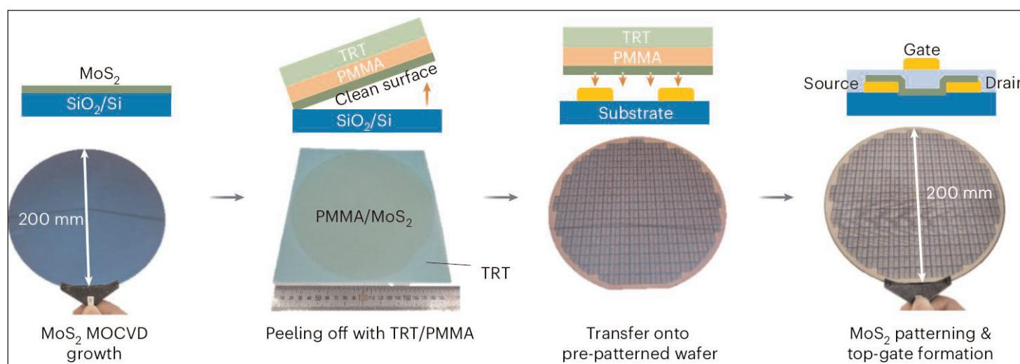
**Figure 1. Simplified 200mm-wafer-scale fabrication process for bottom-contact FET.**
