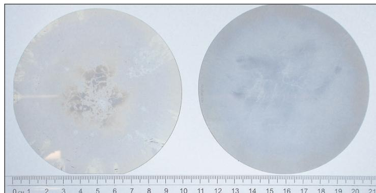
**Comparison of Crystal IS 100mm bulk AlN substrate from Q1/2024 (left) with 90% usable area and Q2/2024 (right) with 99.3% usable area.**
