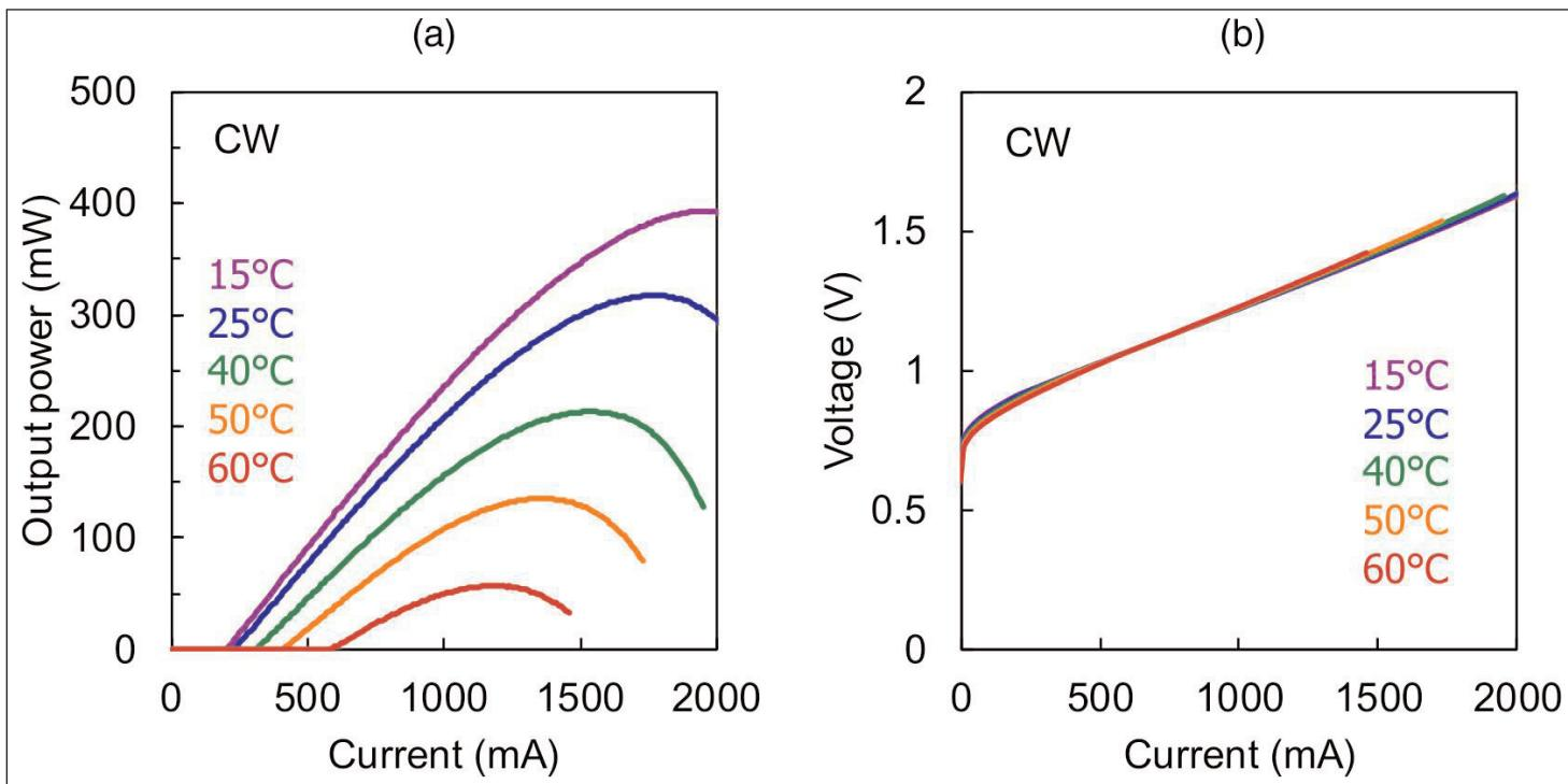
**Figure 2. (a) Light output power-current (L-I) and (b) voltage-current (V-I) characteristics of fabricated 200μm-diameter PCSEL under CW conditions from 15°C to 60°C.**
