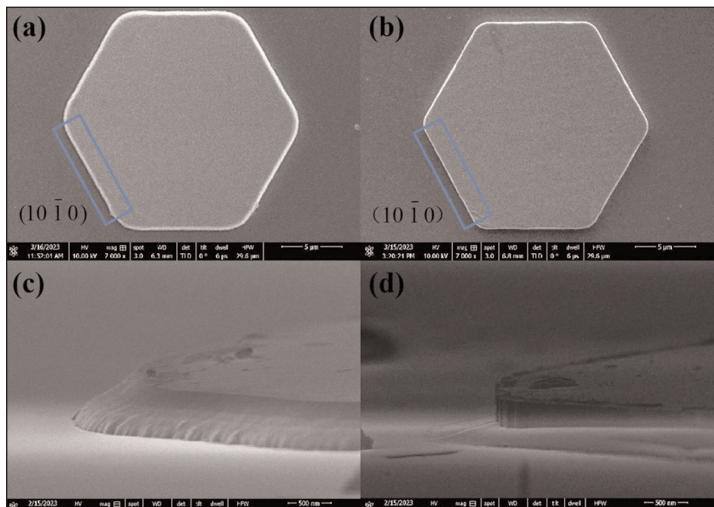
**Figure 2. Scanning electron microscope (SEM) images of 10 $\mu\text{m}$  hexagonal QD LED. Top views (a) before and (b) after TMAH treatment. Bird's-eye views of the sidewall before (c) and after (d) treatment.**
