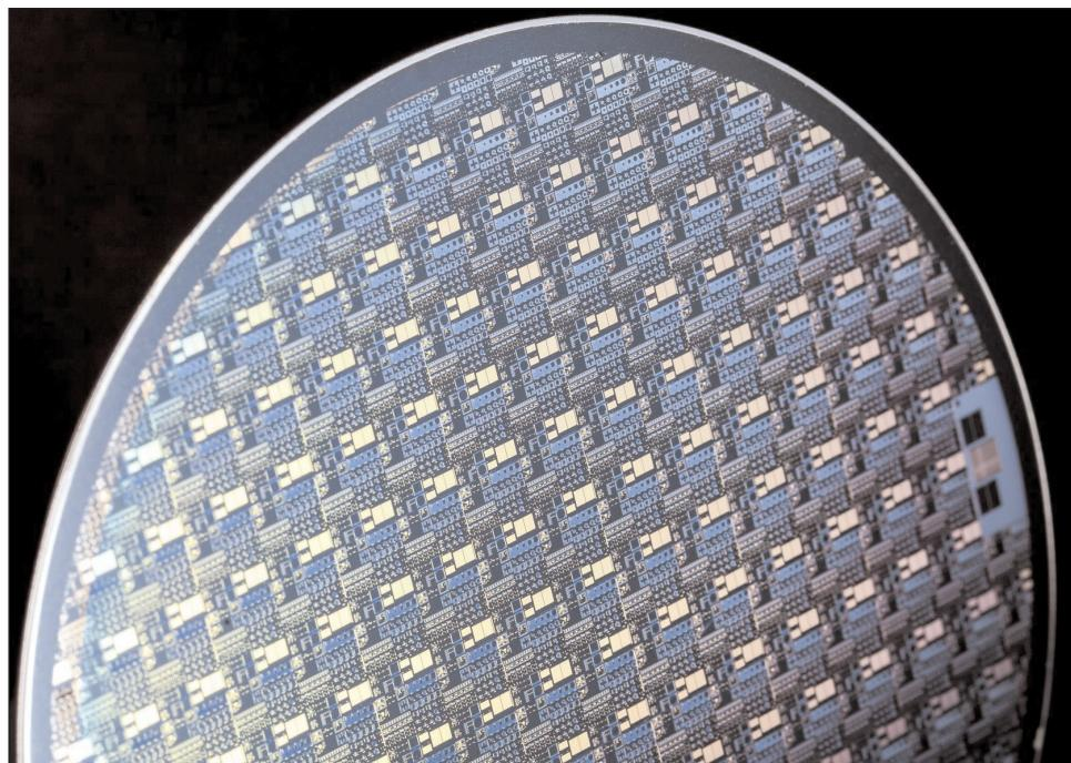
**GaN-on-Si wafer comprising vertical components, developed by Fraunhofer IAF,**
