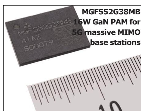
a GaN PAM that achieves an average output power of 8W (39dBm) over a wide frequency range of 3.4–3.8GHz, suitable for 64T64R mMIMO antennas (64 transmitters and receivers) in 5G
