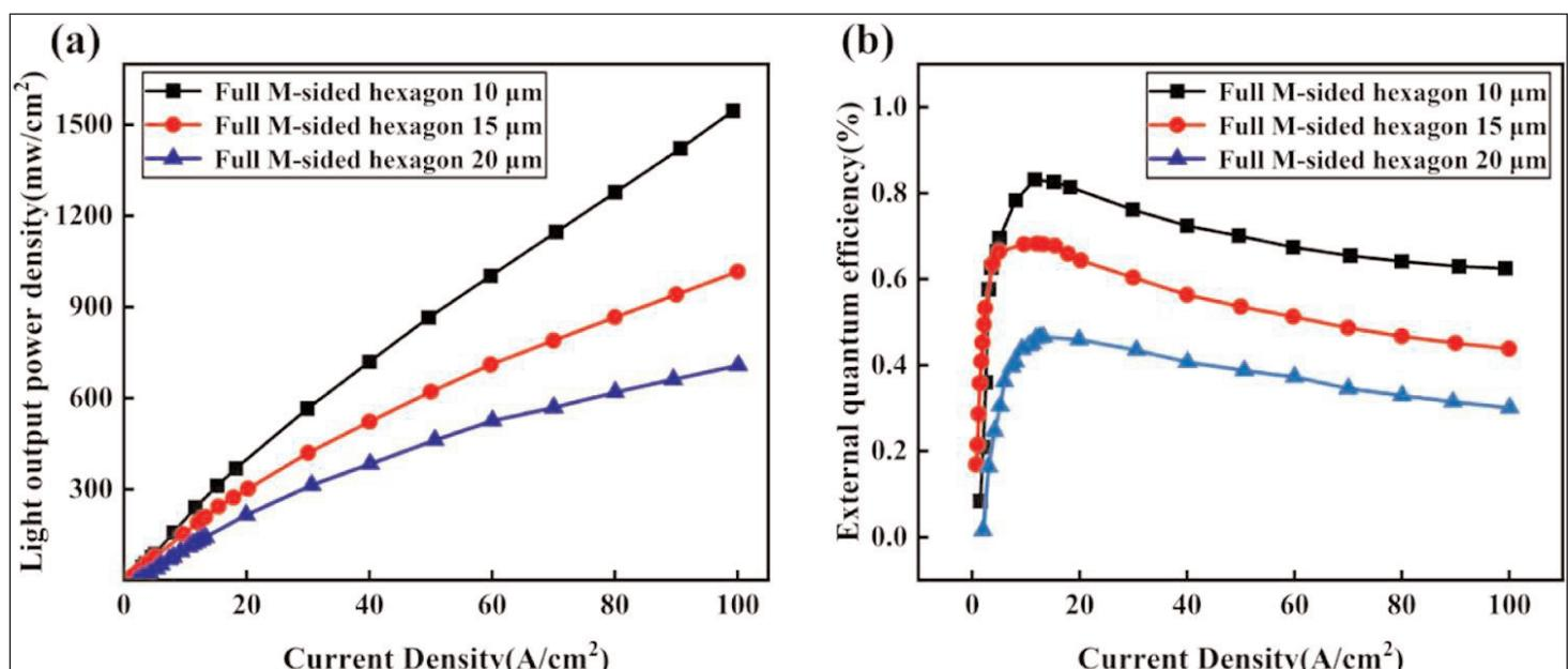
**Figure 3. (a) Light output power (LOP) density and (b) external quantum efficiency (EQE) versus current density for different-sized micro-LED arrays.**
