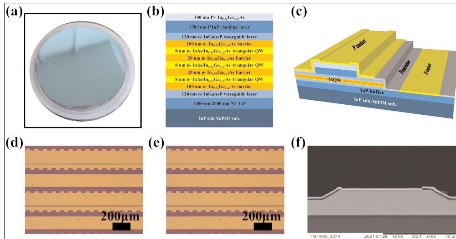
**Figure 1.** (a) As-prepared InPOI substrate; (b) epitaxial laser structure on InP or InPOI; (c) schematic 3D diagram of lasers; optical microscopy images of as-fabricated laser bars on (d) InP and (e) InPOI; (f) cross-section scanning electron microscope (SEM) image of as-cleaved laser on InPOI.
