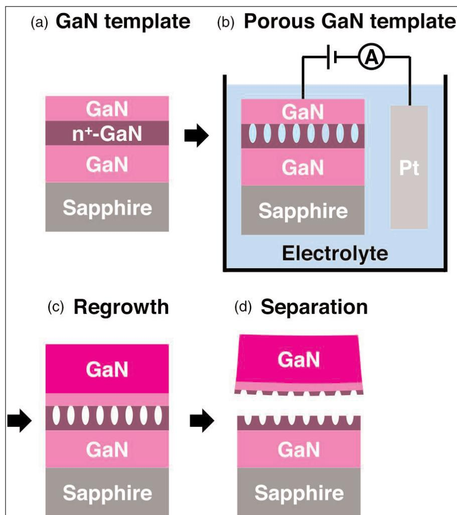
**Figure 1. Process flow: (a) GaN template, (b) porosification by electrochemical etching, (c) regrowth of thick GaN layer by HVPE and (d) separation of free-standing GaN substrate from during cooling after HVPE growth.**
