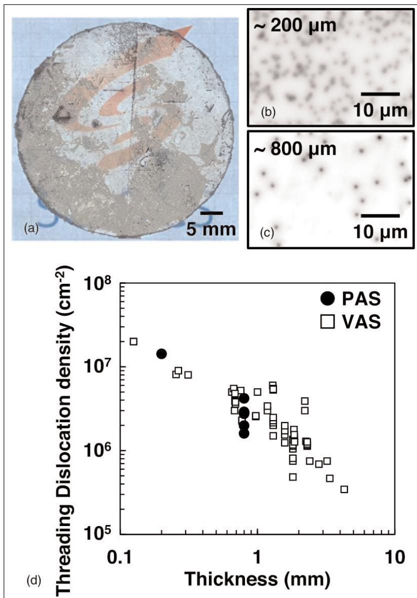
**Figure 2.** (a) Photograph of  $800\mu\text{m}$ -thick GaN layer grown on porous GaN template. Plan-view CL images of (b)  $200\mu\text{m}$ - and (c)  $800\mu\text{m}$ -thick GaN grown on  $20\text{V}$  porous GaN templates. (d) Layer thickness versus TDD values, comparing PAS and VAS separation.
