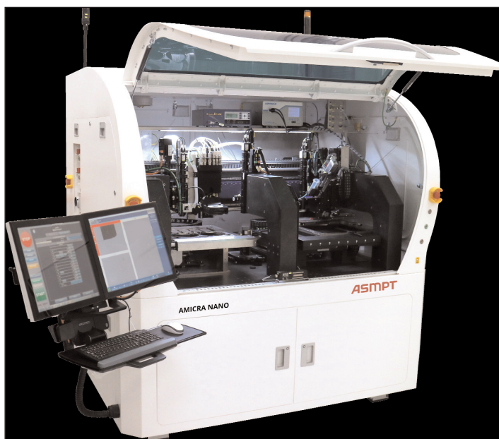
The AMICRA NANO high-precision die and flip-chip bonder.
