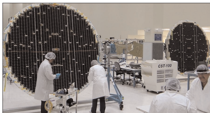
Spectrolab employees work to complete assembly of the Starliner solar panels in Sylmar.
