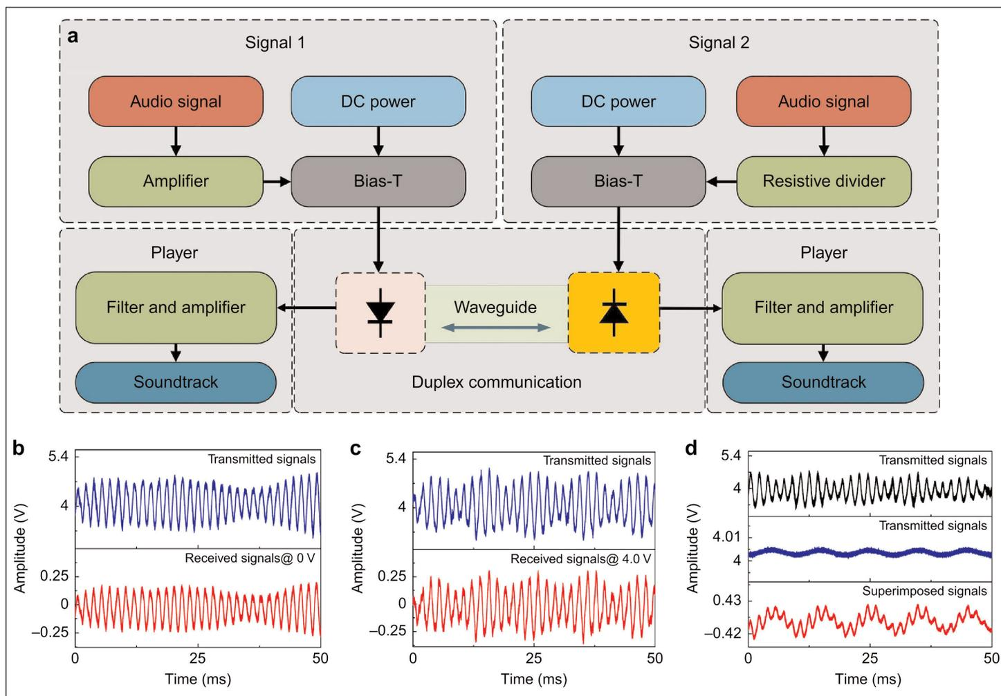
**Figure 2. Full-duplex audio communication using monolithic multi-component system. (a) Schematic. (b) Audio signals received at circular MQW-diode with zero bias. (c) Audio signals received at circular MQW-diode with bias voltage of 4.0V. (d) Superimposed signals under simultaneous emission-detection condition.**
