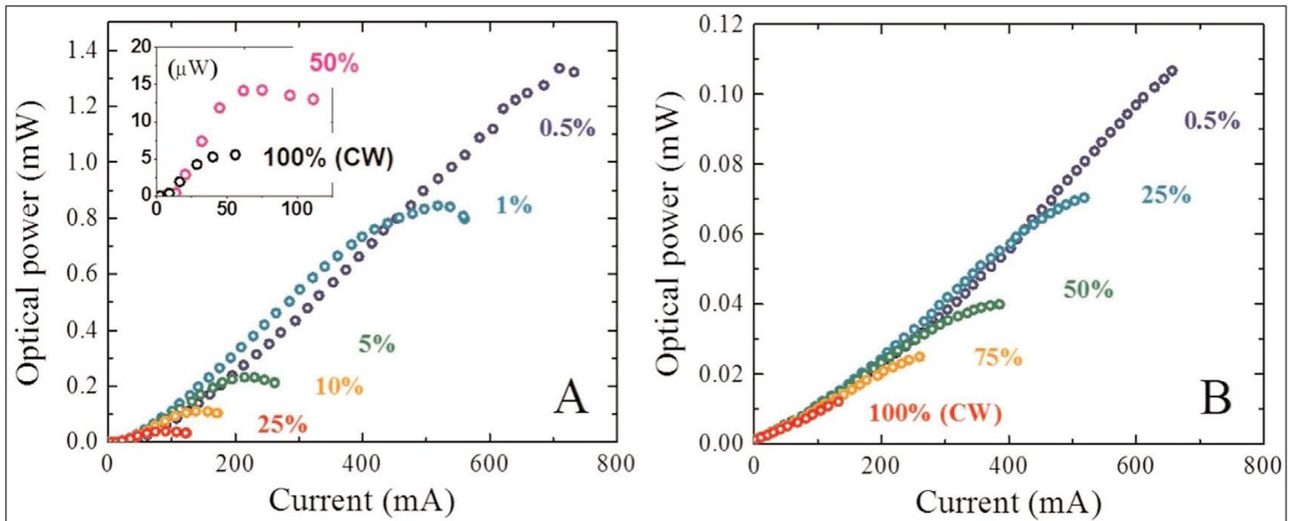
**Figure 8. Optical output power measurements of UV-LEDs grown on silicon (A) and sapphire (B) as a function of injection current for different duty cycles.**
