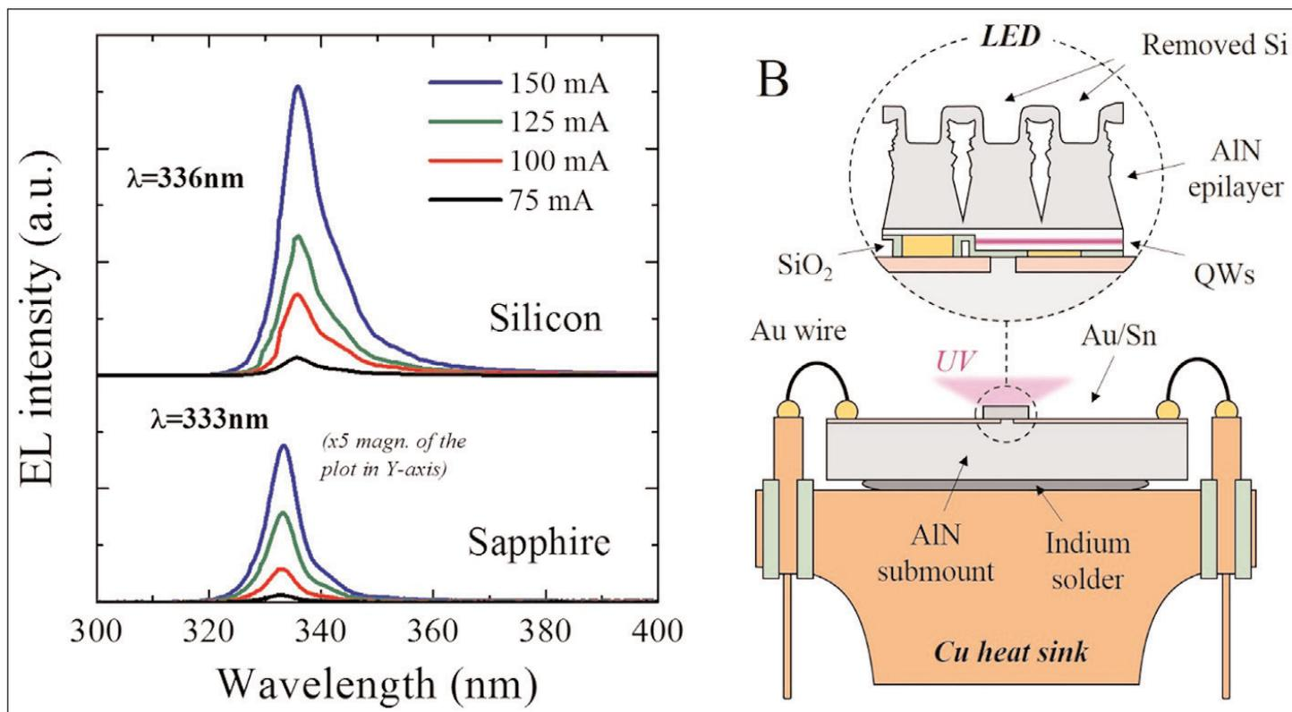
**Figure 7. (A) Electroluminescence spectra of UV-LEDs grown on silicon and sapphire ( $\text{Al}_2\text{O}_3$ ) recorded at different current densities. (B) Schematic of device structure grown on silicon.**
