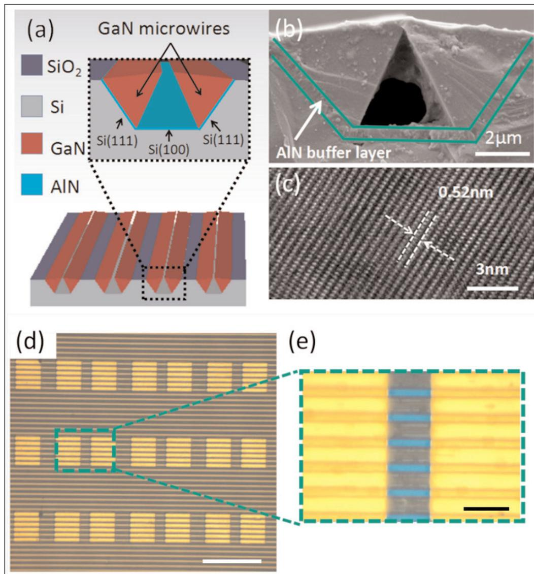
**Figure 5. (a) Schematic of GaN-based microwire arrays on patterned silicon substrate. (b) Typical scanning electron microscope image. (c) High-resolution transmission electron microscope image of GaN microwire. (d) Optical microscope image of fabricated orderly arranged detectors; scale bar 100µm. (e) Enlarged image of one detector; scale bar 20µm.**
