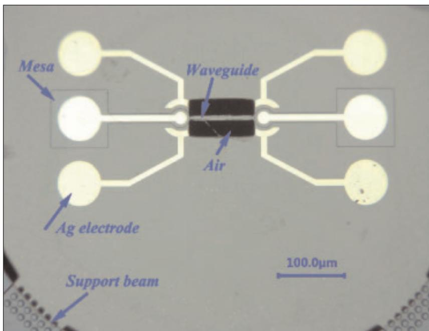
**Figure 4. Optical microscopy image of monolithic multi-component system.**
