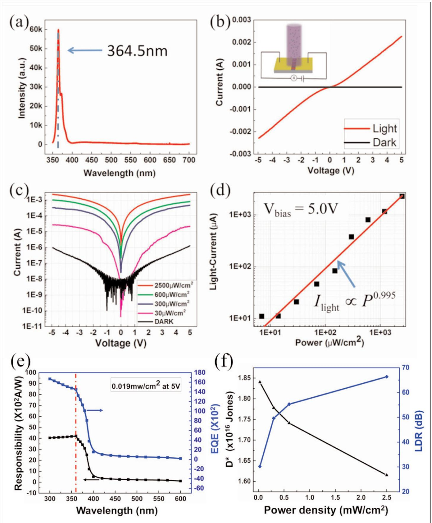
Figure 6. (a) Room-temperature micro-photoluminescence spectrum of GaN microwire. (b) Current-voltage characteristics both in dark (black curve) and under 325nm UV illumination (red curve); inset, testing schematic diagram of photodetector. (c) Light-density-dependent current-voltage curves. (d) Current variation as function of light intensity. (e) Responsivity and EQE-dependent wavelength curves. (f) Specific-detectivity-dependent power density curves.
