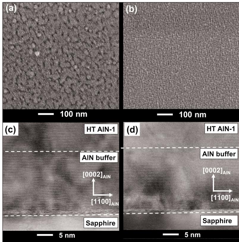
**Figure 1. Surface morphologies of (a) MOCVD AlN buffer and (b) sputtered AlN buffer taken with scanning electron microscope (SEM) using magnification of 300,000. Cross-sectional high-resolution transmission electron microscope (HRTEM) images of (c) AlN film with MOCVD AlN buffer and (d) AlN film with sputtered AlN buffer.**
