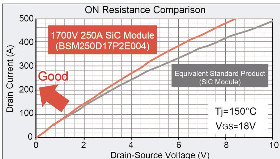
field-effect transistors (MOSFETs) and SiC Schottky barrier diodes (SBDs) into the same module and optimizing the internal structure makes it possible to achieve an ON-resistance 10% lower than other SiC products in its class. This translates into improved energy savings and reduced heat
