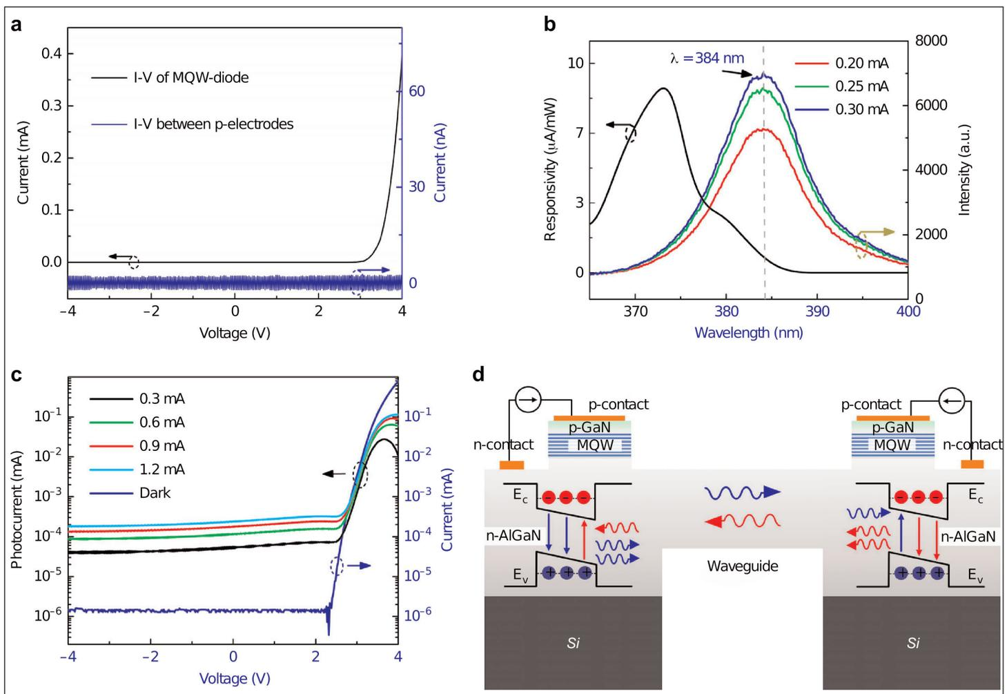
**Figure 1. Optical & electrical performance of monolithic multi-component system. (a) Measured current-voltage I-V curves. (b) Electroluminescence spectra and spectral responsivity of ring MQW-diode. (c) Induced photocurrent at circular MQW-diode as function of injection current of ring MQW-diode. (d) Schematic of full-duplex light communication of monolithic multi-component system using identical MQW-diodes.**
