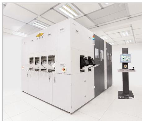
**EVG's GEMINI automated production wafer bonding system for 200mm wafers.**
