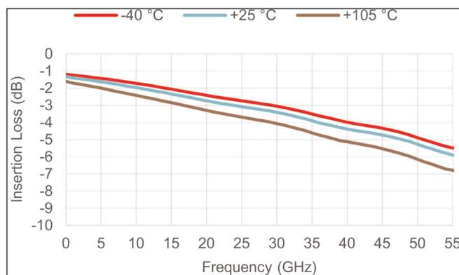
**The PE43508 features low insertion loss across a wide frequency and temperature range.**
