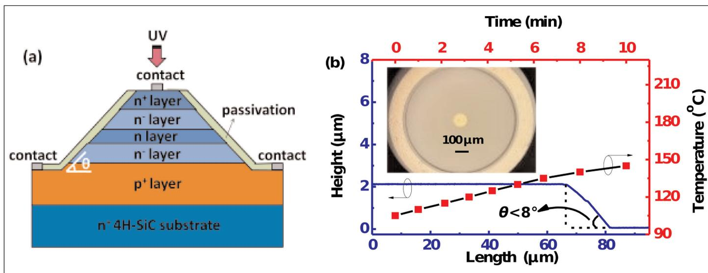
**Figure 1. (a) Schematic cross section structure of 4H-SiC APDs; (b) temperature variation for photoresist reflow technique and profile of beveled mesa and (inset) top-view photo of 800 $\mu\text{m}$ -diameter 4H-SiC APD.**
