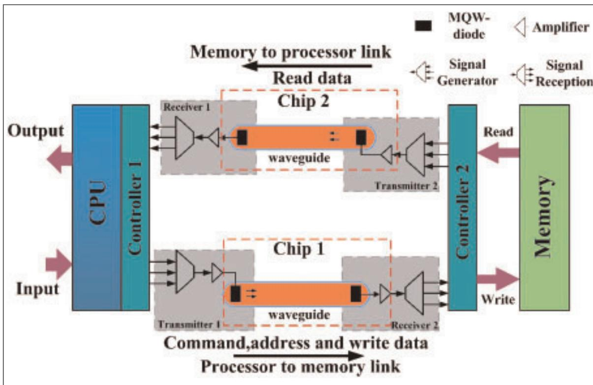
**Figure 3. Schematic of optical communication between processor and memory via monolithic multi-component system.**
