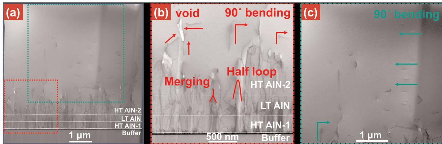
Figure 2. Cross-sectional dislocation distributions of AlN film with sputtered AlN buffer.
