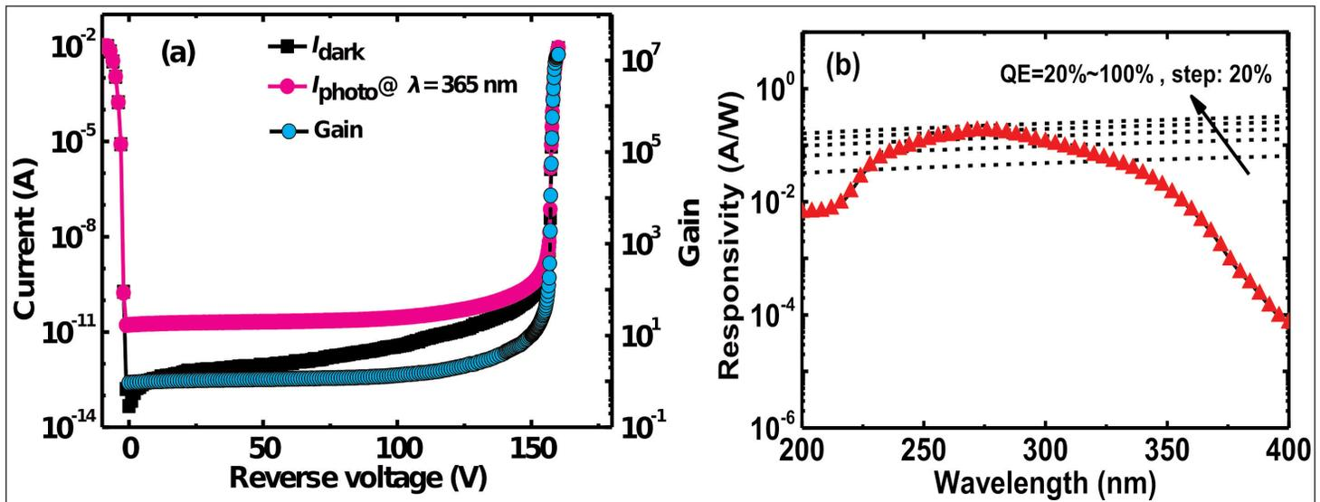
**Figure 2. Ultraviolet detection performance of 800µm-diameter 4H-SiC APD: (a) current–voltage measurements and calculated multiplication gain; (b) spectral response corresponding to unity gain at reverse voltage of 140V.**
