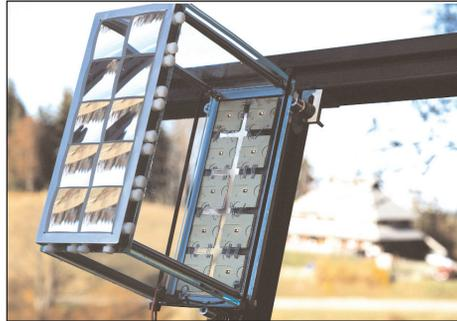
**HCPV module with record 41.4% efficiency.**
