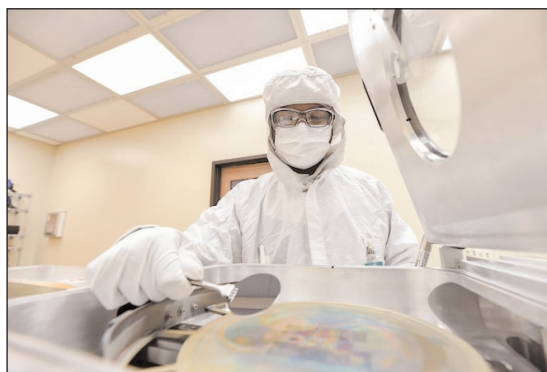
Md. Mehedi Hasan Tanim, a doctoral student of electrical and computer engineering, prepares to grow ScAlN thin films using PEALD. The method can layer ScAlN on 3D structures while previous approaches were restricted to flat surfaces, opening up new opportunities for device integration. Credit: Jero Lopera, Michigan Engineering.
