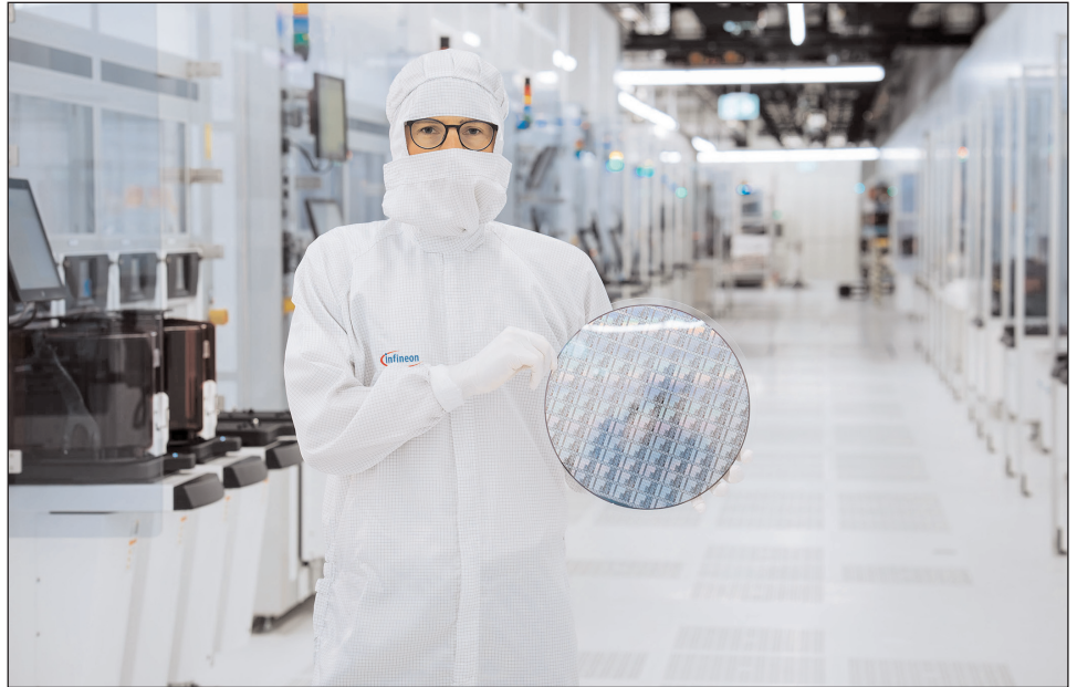
A technical engineer in the cleanroom at Infineon in Villach, Austria, holds a 300mm gallium nitride wafer.
