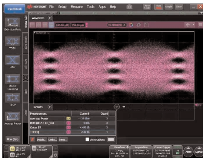
Measured eye at 106Gbaud/s ER=4.5dB, TDECQ=2.4dB.
