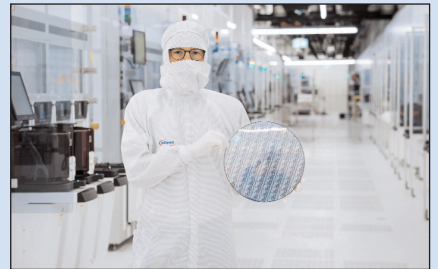
p27 Infineon has piloted the first 300mm power GaN wafer technology on an existing large-scale 300mm silicon line.
