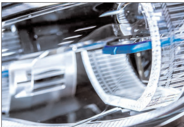
BMW 7 Series headlight with laser light.
