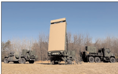
The GaN-based G/ATOR Ground/Air Task-Oriented Radar system.
